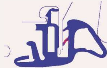
EQUIVALENT CAUCHY STRESS CONTOURS: MOUNT-TO-DOOR FRAME (INCREMENT 17)
