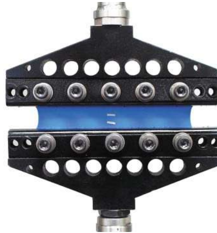
PLANAR SHEAR TEST WITH LASER REFLECTION TAGS
